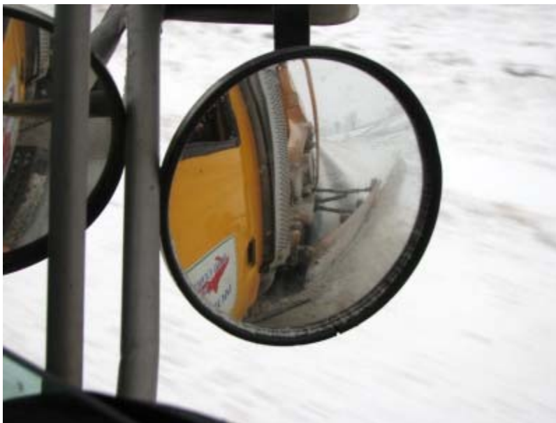
Looking at a convex mirror on the side, snow flies off the wing plow into the ditch.
